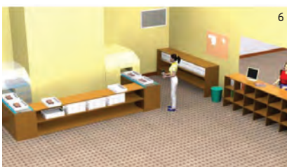
4, 6 ASRS supply and return activities. The library operator retrieves book from tote coming via tote lift, scans it out of system, and hands it to student. For the return activity the library operator places returned books into totes onto tote lift to send back to the ASRS worker for automated storage in the mini-load via SRC 5 ASRS workstation pick and store activities. The ASRS worker picks up ordered book from bin, places it into a tote, and sends it via the tote conveyors to the tote lifts reaching the book station. For the store activity the worker removes the returned book from the tote, places it in the bin, and sends the bin via the in's conveyors to the SRC storing it back in the mini-load racks 7,8 Section and plan drawings showing the ASRS solution within the library architecture
